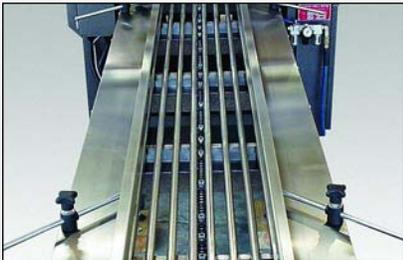
**FFT**-Flighted fall through infeed is ideal for products such as pizza or baked goods that experience drop off of toppings. This design prevents excessive debris build up that would normally contribute to down time during production, and it also minimizes debris in the finished package. This infeed is constructed of stainless steel and is easy to clean. Debris catch trays are also available with this system.
