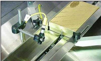
**F-Flighted Pin** Infeed is ideal for narrow products of 1" wide to the maximum width capacity of the wrapper, the quick change pusher pins are ideal for fast spacing changes. This infeed can be extended up to 45' in length for use as an assembly conveyor or mounting of multiple friction feeders and hoppers. Has a maximum pusher height of 2".
