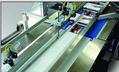
**G-Gated** infeed has a 4' accumulation conveyor, a positive stop product gate, an acceleration conveyor and product pusher pins. It easily adapts to existing production lines. The product is received from the customer's conveyor onto the 4' accumulation conveyor, the product is advanced to the positive stop and placement gate which releases the product in phase with the pusher pins. The product then advances into the film web in phase with the cross seal.
