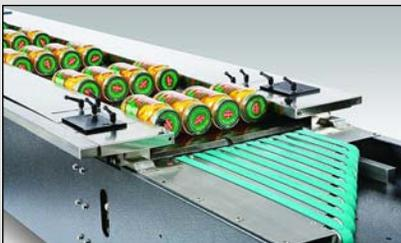
**FB-Flighted Bar** infeed is ideal for multi-packs and odd shaped products, offered in 9 to 18 foot lengths. This infeed features adjustable height pusher bars and multiple product spacing choices.
