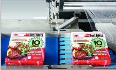
**B-Belt to Belt** infeed easily integrates with existing conveyed production lines. Product is received from existing production line conveyor onto the accumulation conveyor and automatically indexed into the wrapper. System also accepts random length products automatically. **TEACH Programming**, that provides automatic set-up for package length changes, is included.
