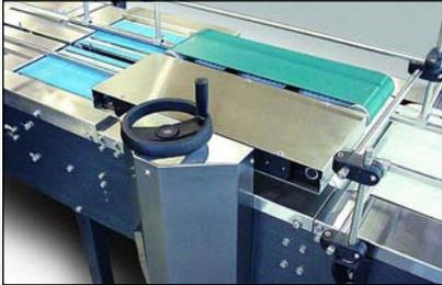
**CBF**-Servo controlled compression belt to flight infeed consist of an accumulation conveyor, a servo controlled compression belt, and flighted pusher pins. Products enter onto the accumulation conveyor and advance into the servo compression belt, that controls back pressure and advances the products in phase with the pusher pins. The pusher pins advances the products into the film web in phase with the traveling cross seal.
